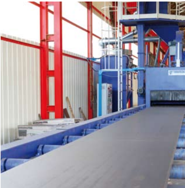
Preliminary sandblasting for all UNIBRIDGE® parts
