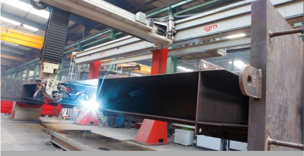
Robot for manufacturing box girders
