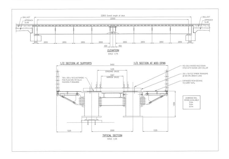
UNIBRIDGE® Rail Solutions have been conceived for temporary railway applications, where a railway bridge needs to be installed very rapidly to replace either a damaged bridge (accident or earth tremor) or an existing bridge under repair or heavy maintenance.
